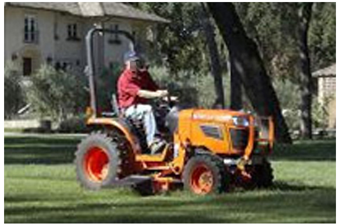
Mower with rollover protection structures.
