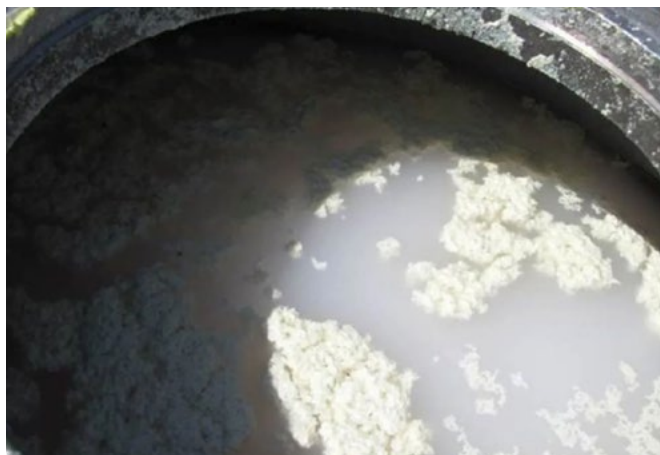
Figure 2. Clumping as a result of over-agitation in the spray tank. (Used with permission from Fred Whitford, Purdue University.)
