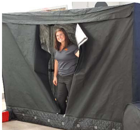
Figure 4. Heat Chambers can be kept on site to treat bed bug infested furniture. (Morgan Wilson, Virginia Tech)
