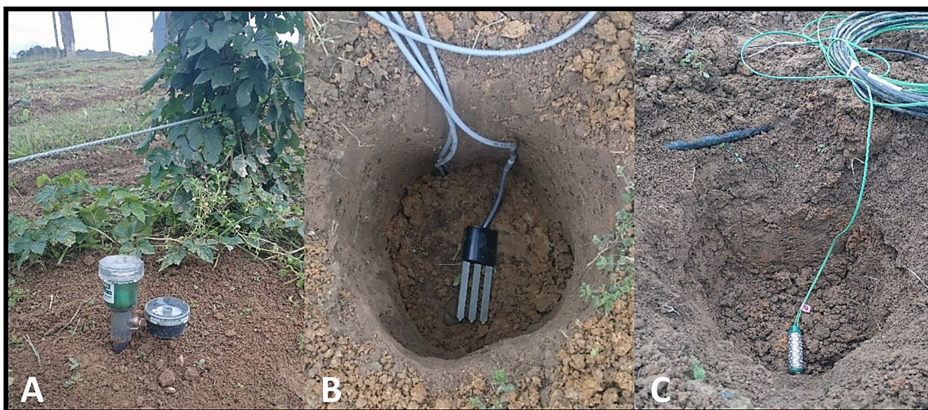
Figure 7. Examples of soil moisture meters used to determine irrigation requirements of hops. A) A tensiometer, which measures the tension created when the soil dries and water is drawn out of the fluid-filled tube through a ceramic cap. B) A time-domain reflector (TDR), which measures the speed and intensity of electrical current transmission between the probes inserted into the soil to determine the soil water volume. C) A granular matrix sensor, which measures the resistance of an electrical signal emitted across a porous (normally gypsum) matrix. (Photos courtesy of Daniel Jackson, Virginia Tech.)
